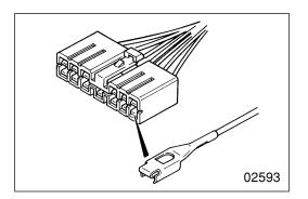
Check for a decrease in contact pressure between the male and female terminals.
