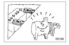
Disconnect the battery terminals before quick-charging the battery.
