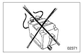
Do not use a high-voltage tester such as a megger for inspection. If a high-voltage tester is used, the diode or regulator might be destroyed.
