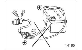
To apply voltage for testing, check that the positive and negative cables are connected properly, then increase voltage gradually from 0 volt. Do not apply voltage higher than the specified value.
