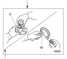
3 10 Impeller-to-water pump shaft interference
