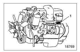
Engine number 1 is punch-marked on the left of the crankcase.
