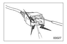
When using testers or the like for continuity tests, be careful not to allow test probes to touch the wrong terminals.
