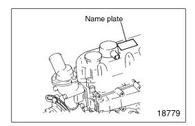
The name plate is attached to the portion shown in the illustration, and indicate the following items.
