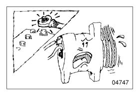
While the engine is running, do not remove the battery terminals. If the battery terminals are removed at that time, a surge voltage is generated and the diode or regulator might be weakened.
